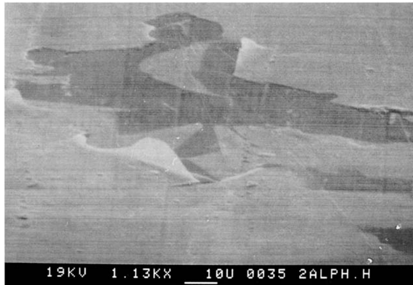
Figure 8 Fracture surface of an adhesive joint treated with a heat-crosslinked electropolymer film.
